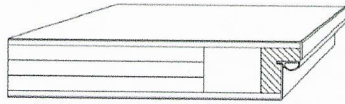
TYPE 43, DOOR THICKNESS APPROX. 43 MM Fire prevention door T30 (E130) Smoke protection door RS (S200) Burglary prevention door RC2 Soundproof door SK37/3 Wet room door
