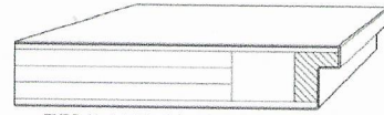
TYPE 40, DOOR THICKNESS APPROX. 40 MM Burglary prevention door RC2 Soundproof door SK32/2
