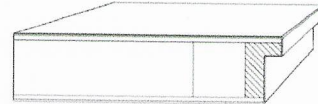
TYPE 50, DOOR THICKNESS APPROX. 50 MM Fire prevention door T30 (E130) Smoke protection door RS (S200) Burglary prevention door RC2 Soundproof door SK32/2 Soundproof door SK37/3
